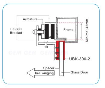
Suitable for use with frameless glass doors .After the door installs with the U-bracket, t he door will become a single swing (inward opening) The diagram shows the **LZ-300** bracket installation instructions.
